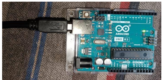
Figure 6: Setting up Arduino and connecting it with laptop via USB.
