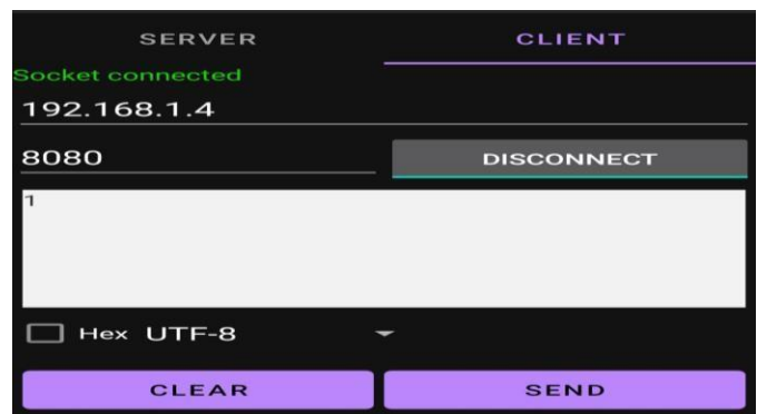
Figure 3: Sending data (1) from mobile through [Simple TCP Socket tester App] over wifi.
