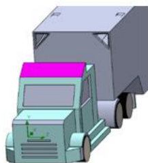
Fig - 6: Combined Venturi passage and Cab roof deflector
