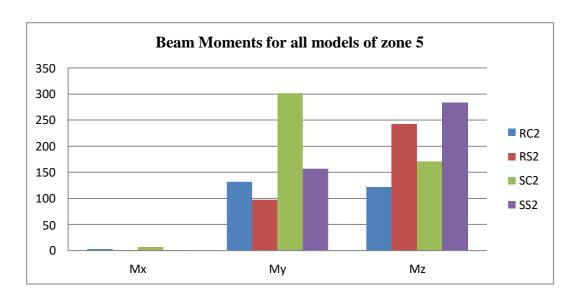
Fig. 5.1.9 Comparison of Beam Moments for all models of zone 5
