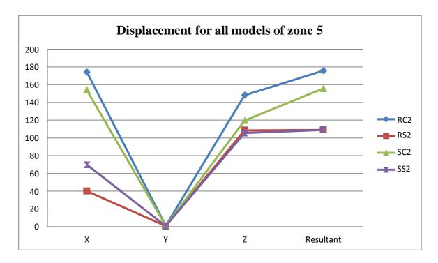
Fig. 5.1.8 Comparison of Displacement for all models of zone 5
