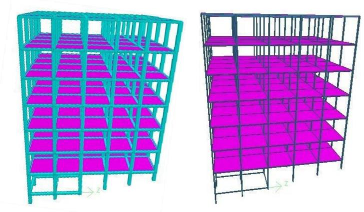
Fig. 4.2(iii) 3D View of RCC sloping building
