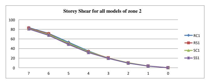
Fig. 5.1.5 Comparison of Storey Shear for all models of zone 2
