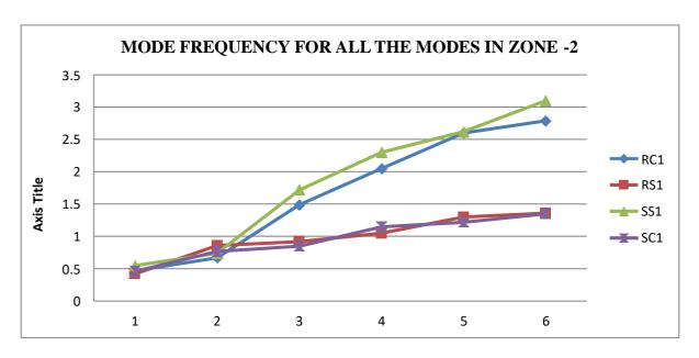
Fig. 5.1.2(a) Comparison of mode of frequency for all models of zone 2
