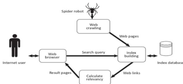
Fig -3: SerpAPI working flowchart
