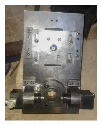
Fig -4: Finish fixture without Component
