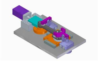
Fig -2: Rough Drilling Fixture
