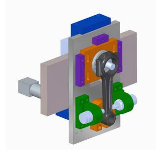
**Fig -3**: Finish Boring Fixture
