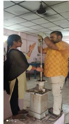
Preparation Of Bituminous Mix Mould
