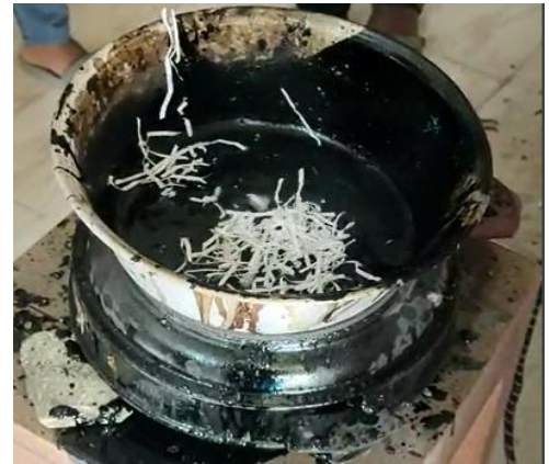
Fig -2: Mixing of shredded plastic and bitumen
