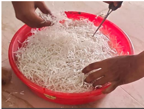
Fig -1: Shredding of HDPE plastic
