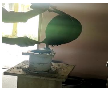
Fig -3: Filling the Marshall compaction mould with the prepared mixture
