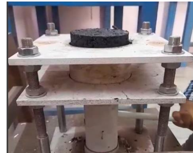
Fig -4: Extraction of specimen from the mould
