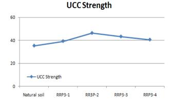
Fig. 3 Unconfined Compression Test on natural soil & RRP3 samples
