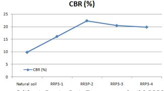
Fig. 4 California Bearing Ratio Test on natural soil & RRP3 samples
