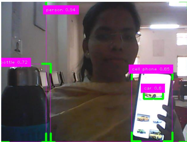
Figure 11 : Cellphone and Bottle detection by using Yolo
