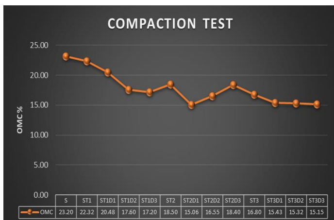
Chart -6: Comparison of OMC values of soil with Stabilized soil (BC Soil +Terrazyme +F Fly ash)
