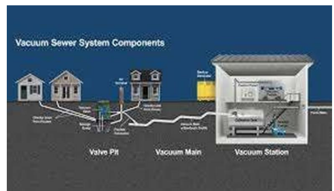
Figure vacuum Sewerage System
