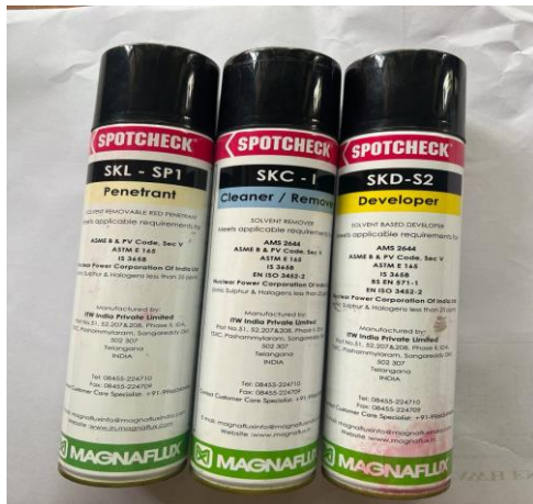
Fig 12: Liquid penetrant testing cleaner, penetrant And developer
