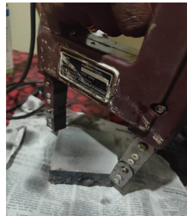
Fig 22: Magnetic Particle Inspection
