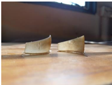
Fig. 5 Curved Trapezoidal winglet vortex generators
