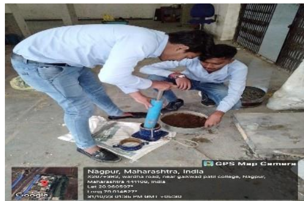
Fig: 7. Proctor Compaction
