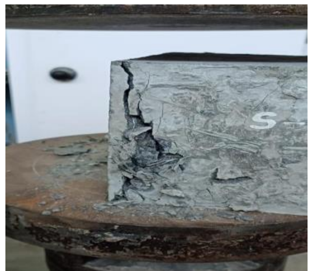
Figure-2: Cube after application of load
