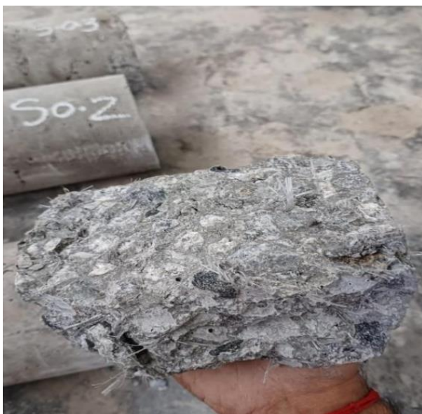
Fig-3: concrete specimen incorporated with TMF fiber showing comparatively less porous
