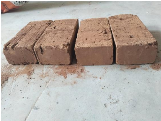
Figure-3: Manufactured clay bricks with sludge and iron tailings
