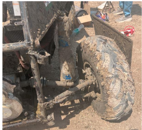
Photograph -5: Rear Suspension System after successful completion of Endurance Race
