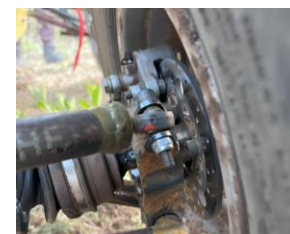
Photograph -3: Actual Rod end failure as predicted from analysis from 2.4
