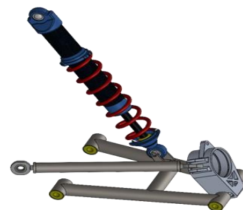
Fig -1: H-Arm Suspension System with Single Upper Lateral Link
