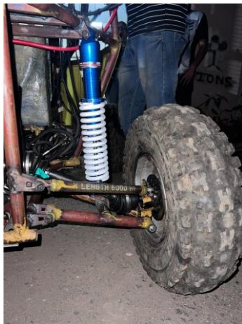
Photograph -4: Rear Suspension System before Endurance Race
