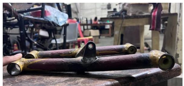
Photograph -2: Actual H-Arm bend after vehicle testing as predicted from analysis from 2.3
