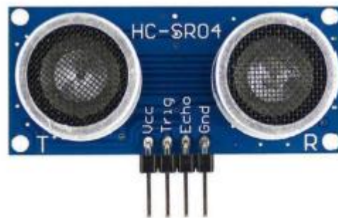
Figure 2: HC-SR04 Ultrasonic Sensor Structure
