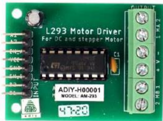
Figure 4: Motor Driver L293 Module Structure
