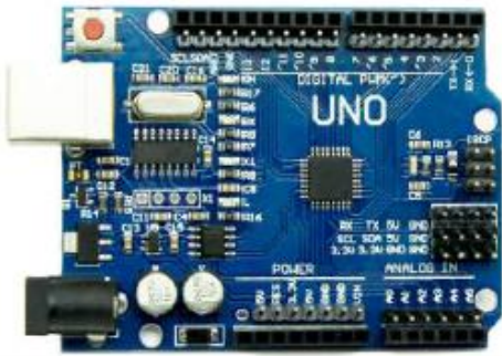
Figure 3: Arduino-UNO ATmega328P microcontroller structure
