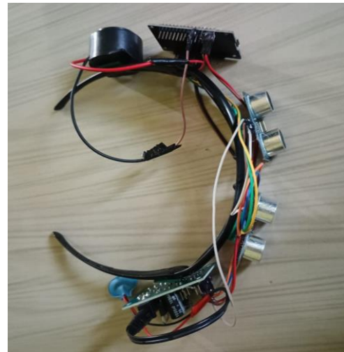
Figuer -4: Ultrasonic smart glass for visually impaired people
