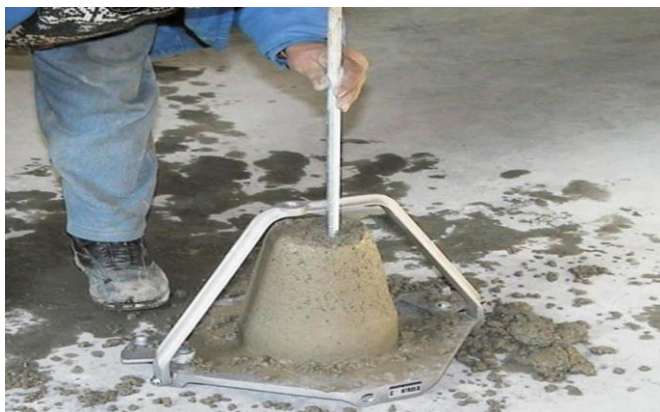
Fig -5: Performing Slump Cone Test
