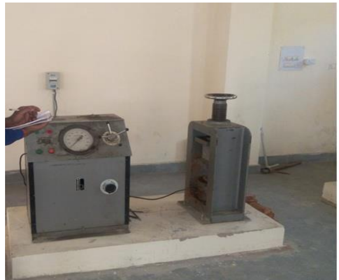
Fig -4: Performing Compressive-Strength Test
