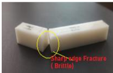
Figure: 7 Impact fracture sample
