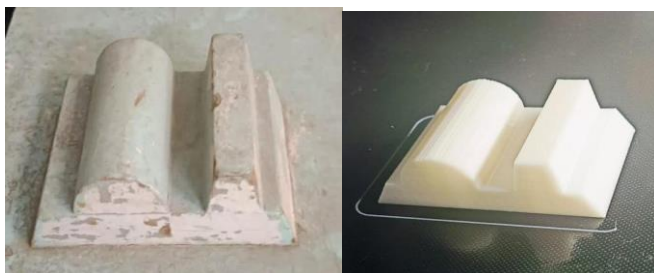
Figure 8 shows that pattern (a) Teak wood pattern and (b) 3D printed PLA pattern
