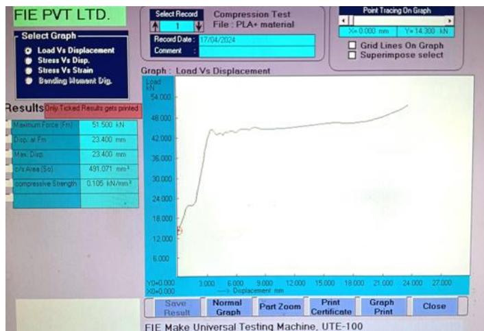
Figure: 6(a) Prepared sample for compression test (b) Dimension of specimen (c) Graphical representation of compression test.
