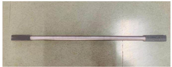
Fig:- 6 Torsion Testing Specimen of material AISI 4130
