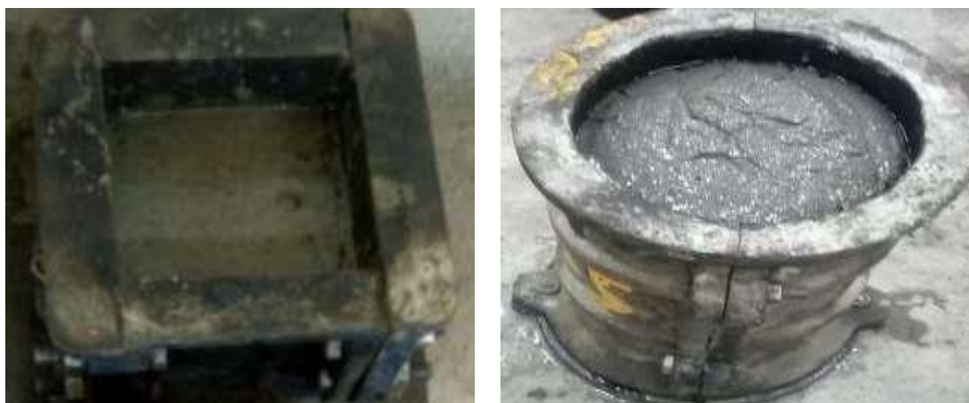
Figure 3 Concrete after filling mould
