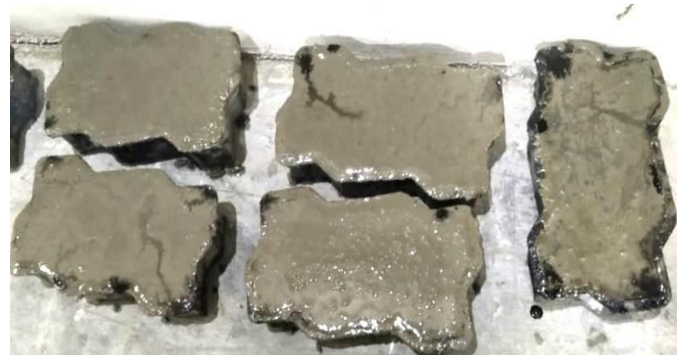
Figure 2: Casting of paver blocks
