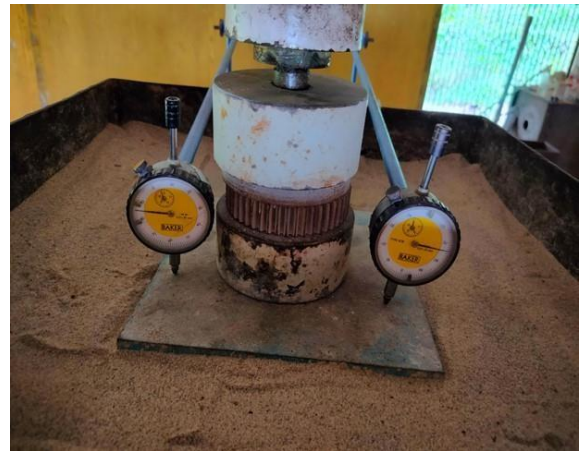
Fig – 4: Plate load setup before loading
