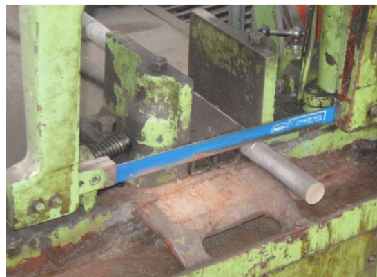
FIGURE: 1 Cutting of work piece with power saw
