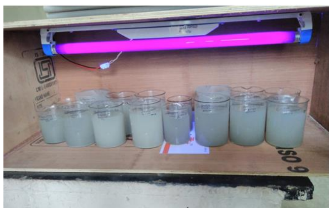
Figure 1: Samples kept under the box for UV light exposure
