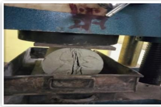
Fig- 3: Split tensile strength test in UTM
