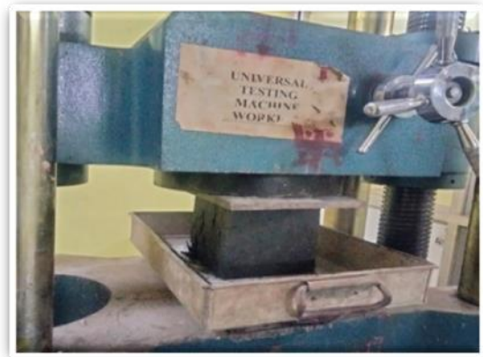
Fig-2: Compressive strength test in UTM
