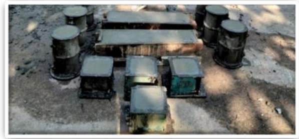
Fig-1: Casting of Cube, Beam & Cylinder
