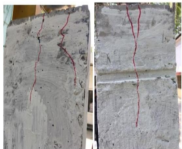
Figure 6 Crack pattern of CS
