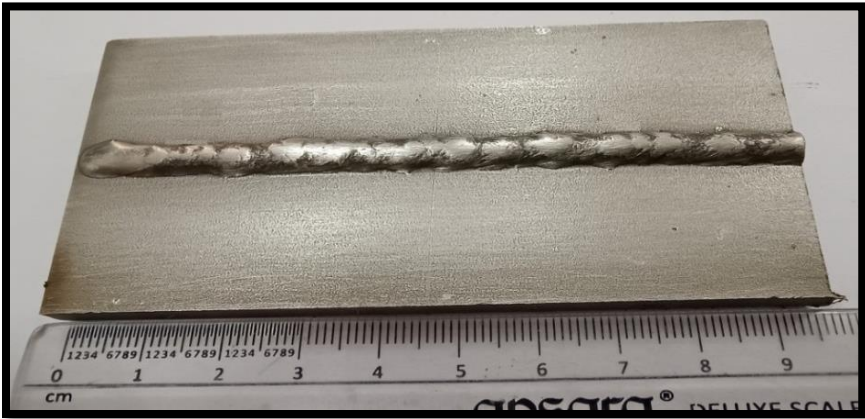
Figure 7 Visual inspection of Sample D, which is free from surface defects
