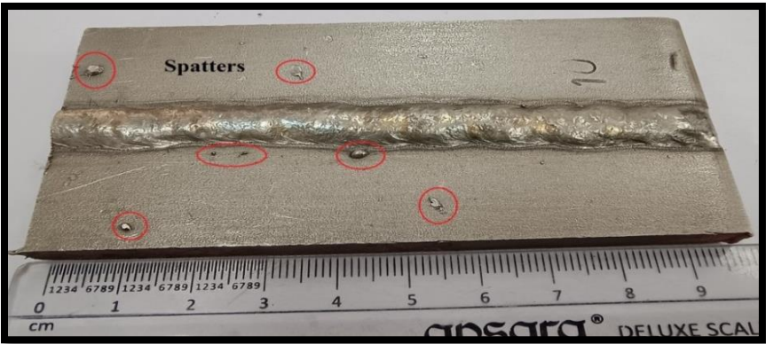
Figure 8 Visual inspection of Sample 10 revealing spatters
