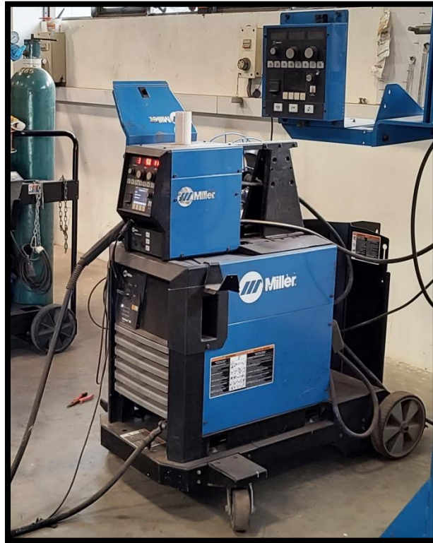
Figure 1 Miller make: Pipe Worx 400 welding power source
