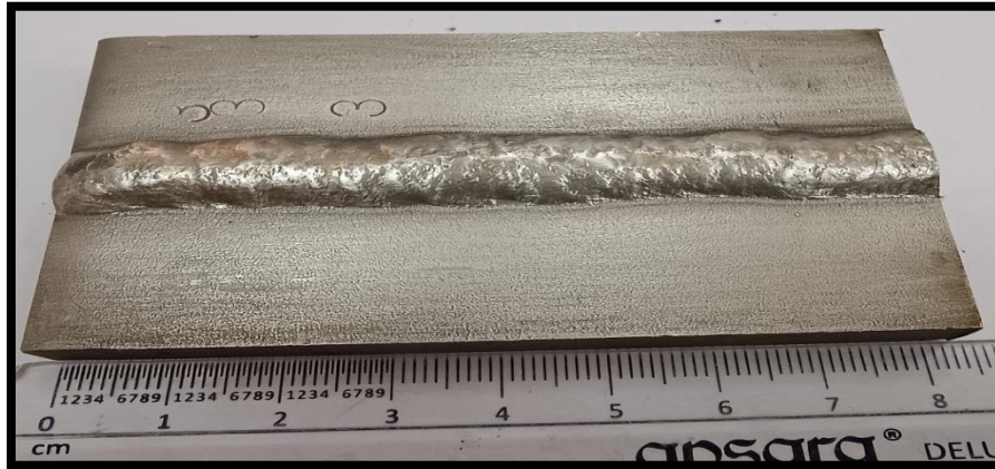
Figure 9 Visual inspection of Sample 3, which is free from surface defects
