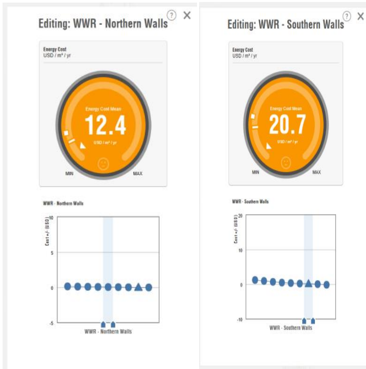
Figure 12: Window-wall ratio (North, South)
