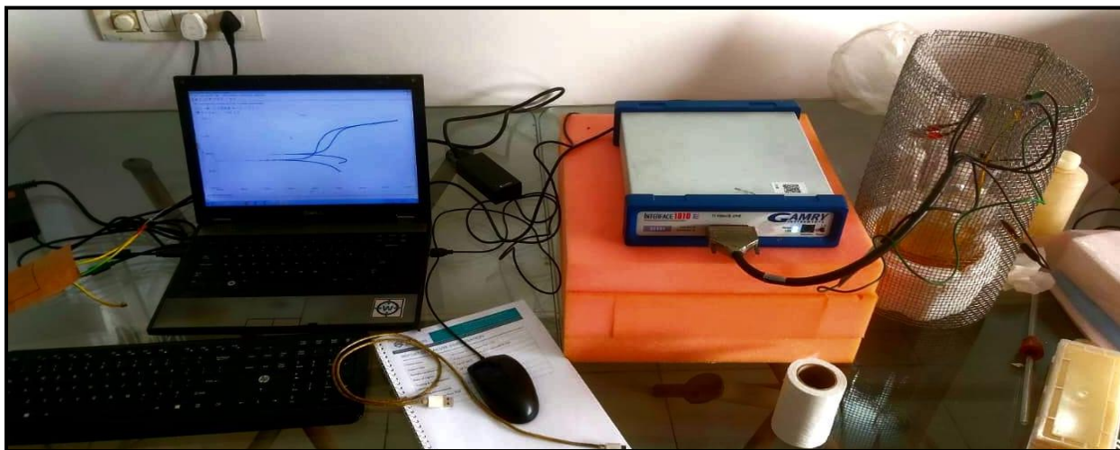
Fig.2 Experimental Setup of Potentiodynamic Polarization Technique
