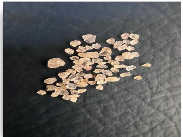
Fig -11: Quartz Particles (Having mean particle diameter of 0.46mm)
