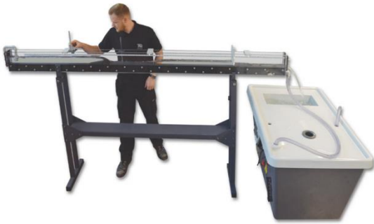
Figure 1: A 2.5 m long flow channel along with hydraulic tank
