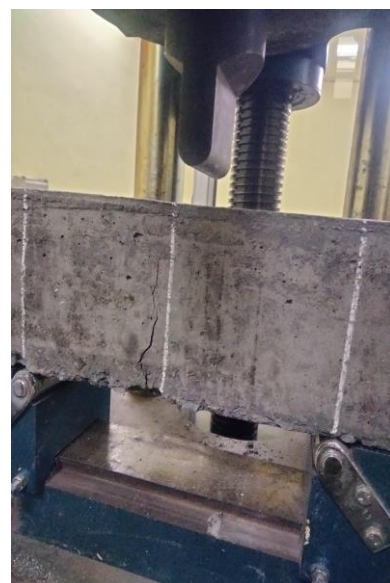
Fig-4: flexural strength test in universal testing machine.
