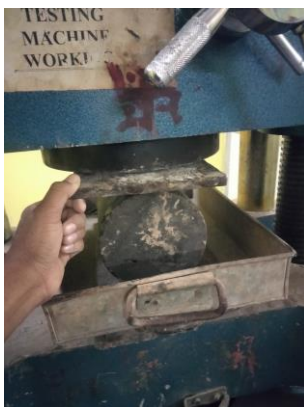
Fig- 3: Split tensile strength test in Universal testing machine.
