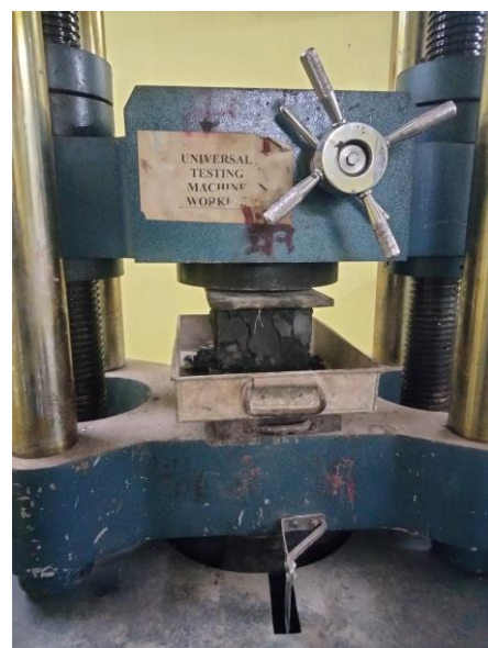
Fig-2: Compressive strength test in universal testing machine.
