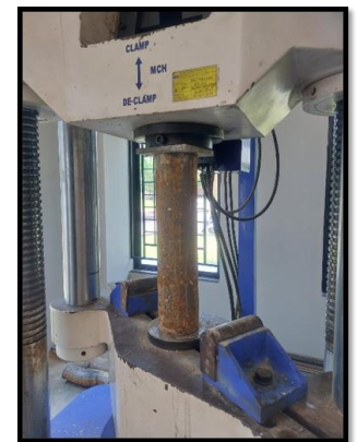
Fig -1: Test set up on UTM
