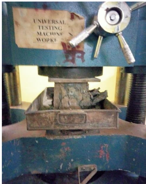
Fig-4: Compressive strength test in UTM
