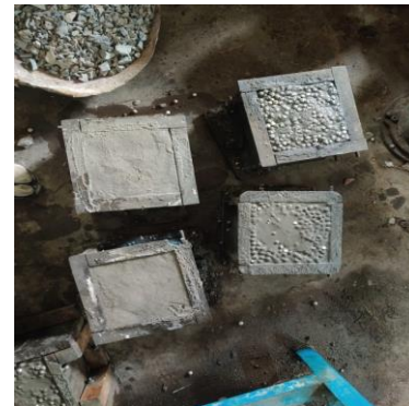
Fig-3: Casting of Cube.
