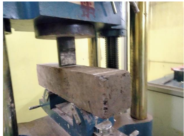
Fig-6: flexural strength test of concrete in UTM
