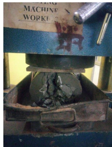
Fig- 5: Split tensile strength test in UTM
