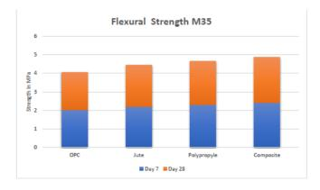
Fig -3.2 Value of Flexural Strength M35
