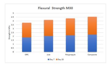
Fig -3.1 Value of Flexural Strength M30
