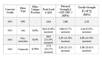
Table -3.4: Flexural and Tensile Strength of M30 on day 7
