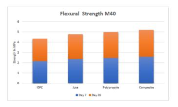
Fig -3.3 Value of Flexural Strength M40
