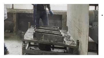
Fig -2.5 vibrating table
