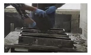
Fig -2.4: Filling molds in 3 layers
