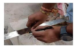
Fig -2.8 50 mm overhang on each side
