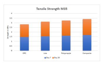
Fig -3.5 Tensile Strength M35
