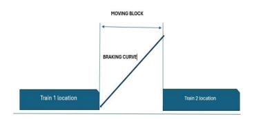
Fig -4: Moving Block Working
