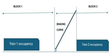
Fig -3: Fixed Block Working
