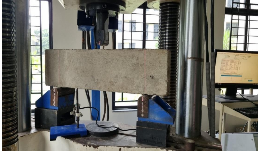
Figure 2 Testing of RC beam section for three-point loading in UTM
