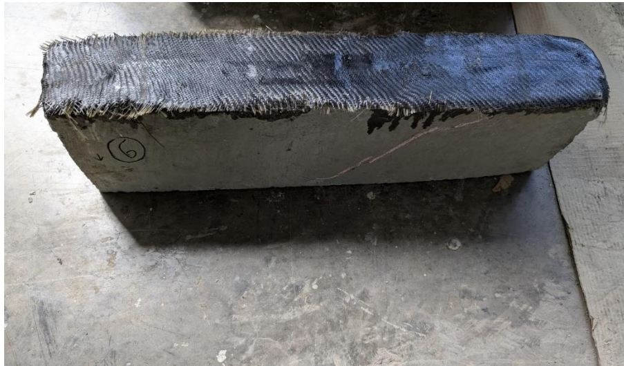
Figure 9 The RC Beam with BFRP fabric @ two sides face only
