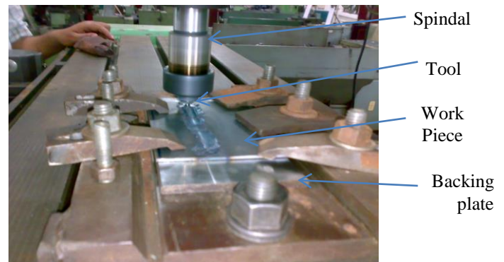
Fig. 1.1 Fixture used in FSW process
