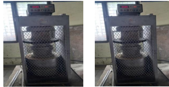
Fig. 1. Compressive strength of concrete cubes
