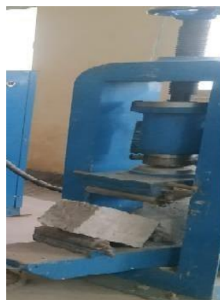
Fig:-3 Flexural Testing Machine Fig:-4 Flexural Strength
