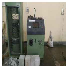
Fig:-1 Compressive Testing Machine Fig:-2 Compressive Strength
