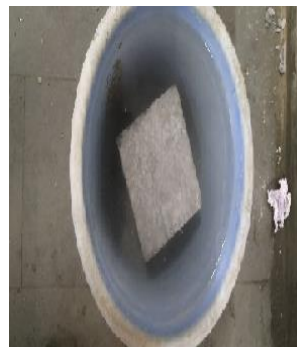
Fig-8 Sample Fully Submerged In Acid Solution
