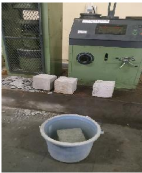
Fig-8 Sample Fully Submerged In Acid Solution
