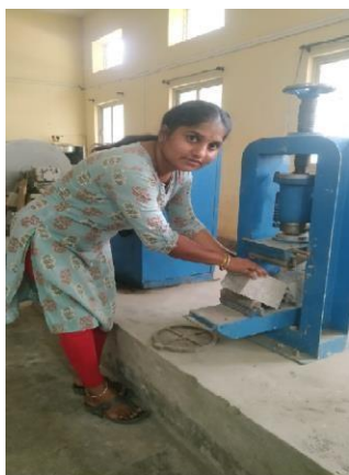
Fig:-3 Flexural Testing Machine Fig:-4 Flexural Strength
