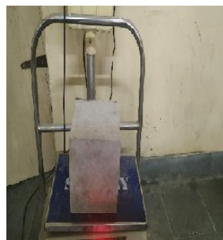
Fig;-6 Initial Mass of the Sample
