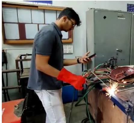
fig5: electric arc welding
