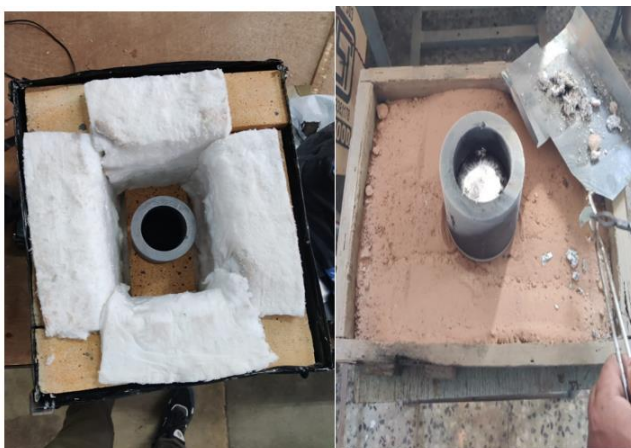
Fig6: Crucible, insulation, molting process
