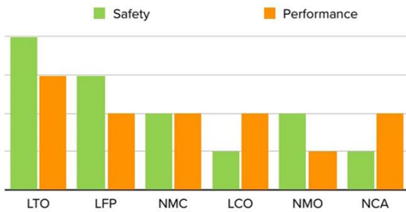
Fig- 4: Comparison of safety and performance of different Li-Ion batteries [4]
