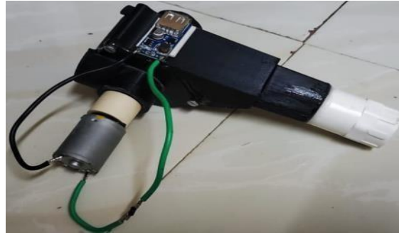
Fig-14: Designed Tesla turbine Prototype.
