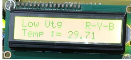
Fig.11. under voltage fault detection on LCD display
