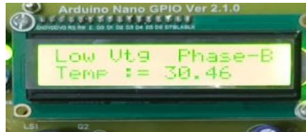
Fig.13. Single phasing fault detection on LCD display
