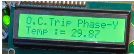
Fig.12. Over current fault detection on LCD display
