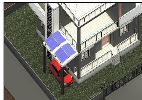
Fig. 17: - Solar power system Revit design
