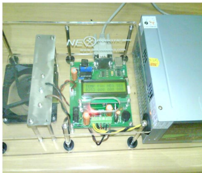
Fig.2. Single Board Heater System
