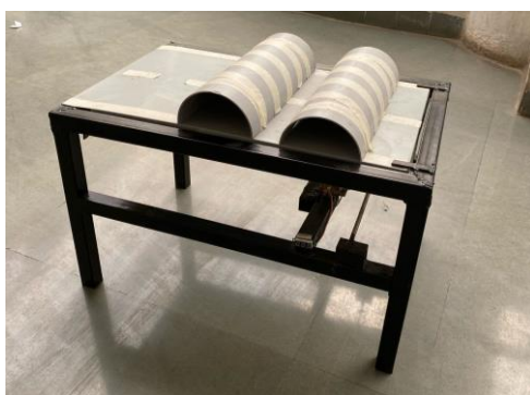
Fig. -12: Assembly of Speed Breaker Mechanism
