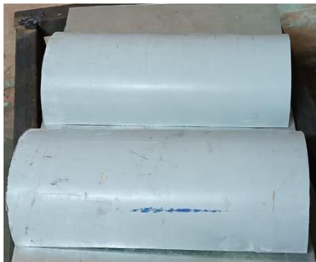
Figure 10 Semicircular Rollers of PVC
